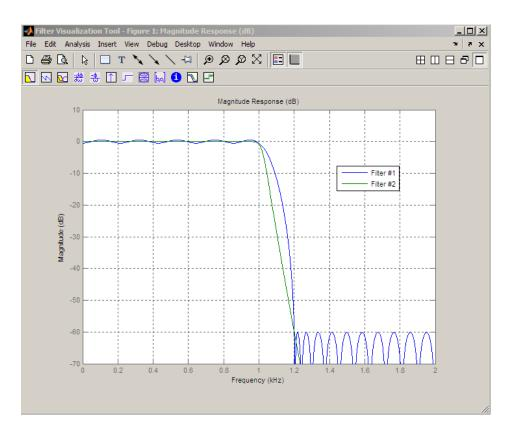
To determine which filter design methods are available for a given Filter Specification Object, use designmethods. For the lowpass filter example above, you have a choice of two FIR and four IIR digital filter designs:
